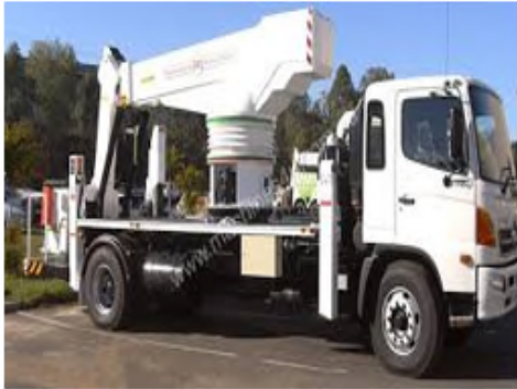
Truck Mounted EWP
